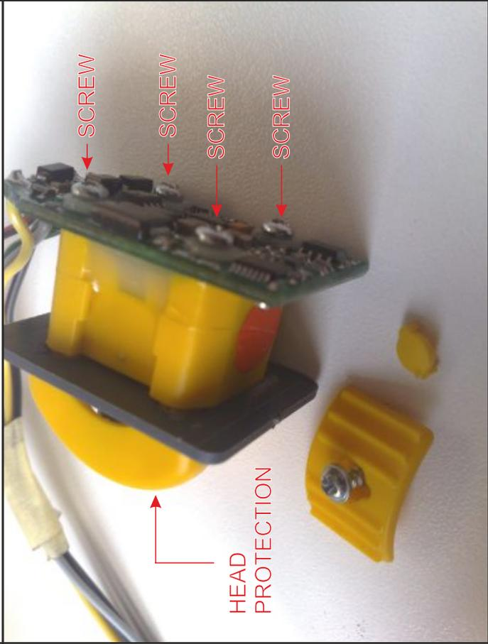
STEP 5: FIX THE HEAD PROTECTION SCREWING THE 4 LOWER SCREW
