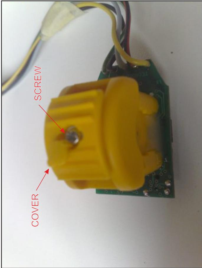
STEP 1: REMOVE THE COVER TO SHOW THE SCREW
